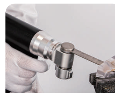
Surgical guide resin toughness test
